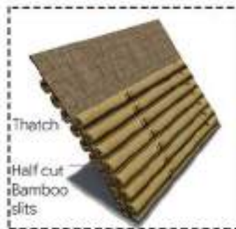
Sandwich slit panel for Waterproofing
