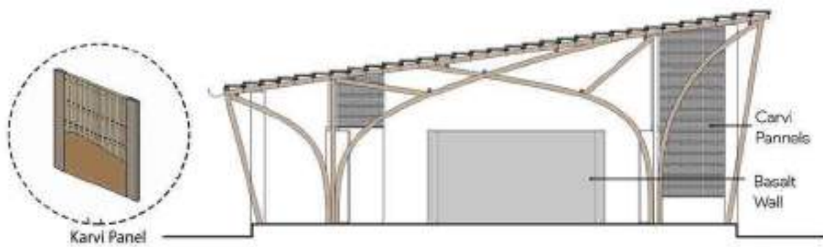
Section through training and workshop space Plinth 1= Ml +0.3m, Basalt Parapet= Ml +0.9m, Wall height (left)= Ml +3.3m, Wall Height (right)= 4.6m
