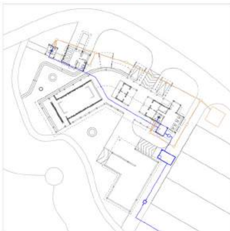
Fig. 67. Water Supply and Drainage Layout
