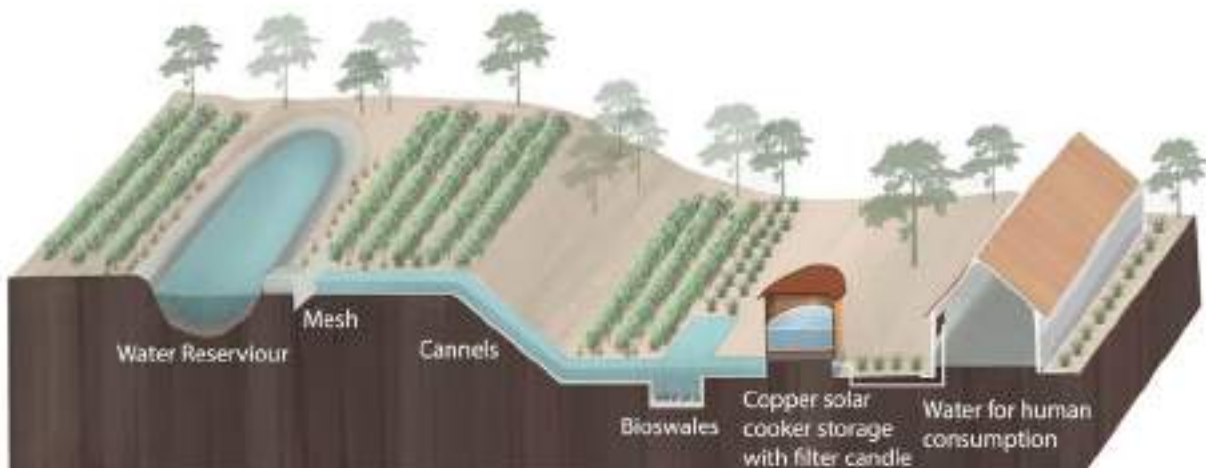
Fig. 80. Water purification supply system
